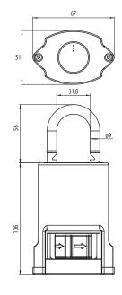
It is very important to push the shackle firmly when closing this will guarantee the padlock is correctly sealed
